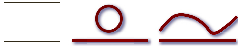
Figure 2. Progression from Casimir’s original configuration of perfect parallel plates, to realistic experimental configurations with different geometries and imperfect surfaces. Here vacuum polarization is probed by the boundaries.
